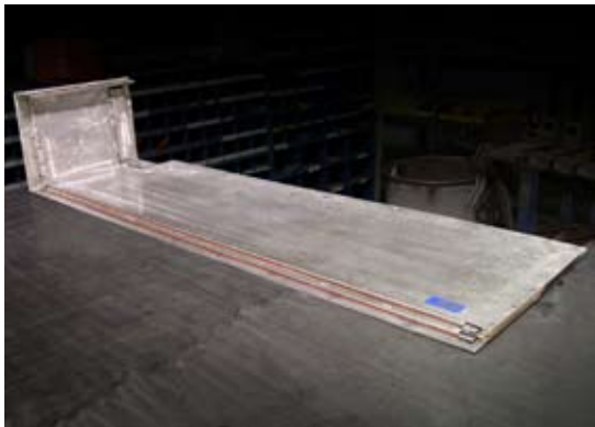
Way cover after repair and refurbishing by Hennig, Inc.
